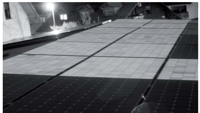
Electroluminescence image to detect allied solar modules
