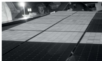
Electroluminescence image for detecting a module string
